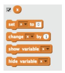
The checkmark means to display the variable on the left side of the stage (where the cat is) and it is the same as clicking the command SHOW VARIABLE. The first two on the left are very important and we will use frequently. The first one called SET assigns a number to the variable (because you don't always want to bother the user to type it in). The second one called CHANGE will be used when we learn to add the numbers from 1 to 100.
