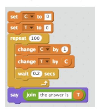
The C variable is the COUNTER. It is set to ZERO to begin and each time thru the loop it increases by 1.
